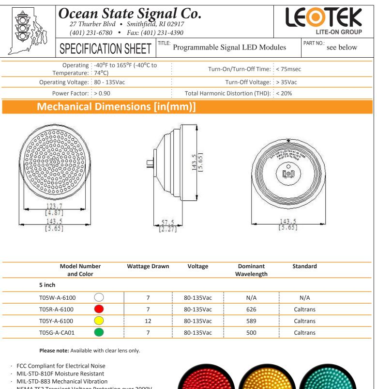
NEMA TS2 Transient Voltage Protection over 2000V
