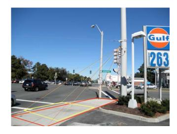
**MigmaIntersection**<sup>TM</sup> is an outdoor passive pedestrian detector with interface to APS pushbuttons for automated locator tone triggering and pushbutton actuation. Using this detector, APS locator tone is silent unless pedestrians are within 12 ft from the signal pole. Based on the presence of pedestrians, APS or mechanical pushbuttons can also be automatically actuated.
