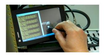
**MigmaMonitor**<sup>TM</sup> is a 7" portable touch-screen monitor. Using the VGA connector, it can be used to monitor the system operation status. Using the stylus pen and on-screen keyboard, one can use this monitor to configure the system for
