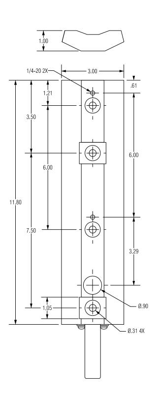
This spacer is designed to offset two Navigators on a 4.0" diameter pole so that two 9" x 12" or 9" x 15" signs can be mounted without conflict. One adapter is needed behind each Navigator. The adapters can either be strapped or bolted to the pole. For bolting, holes are provided to match 6" spacing of most push button signs or spacing for PELCO 5" x 7" frames if these types of frames were previously mounted.
