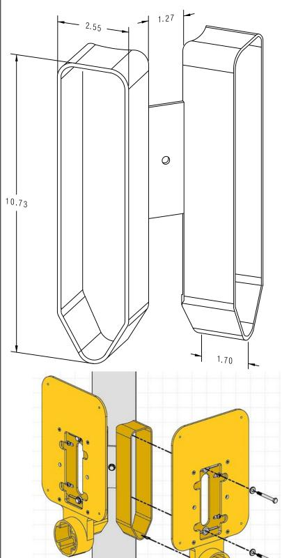
This spacer is designed to offset two Push Button Frames on a 4.5" diameter pole so that two 9" x 12" signs can be mounted without conflict. One spacer is used to mount two Push Button Frames. The spacer is held to the pole by a bolt in the center and the frames mount to the pole with 3" long bolts through the spacer.
