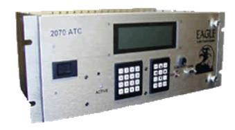
EAGLE now offers its versatile SE-MARC Master Closed-Loop Software on the 2070ATC controller unit, allowing one model of controller to serve as either a master controller or a local controller.
